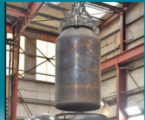
Vitrified waste containers are four feet in diameter, seven feet tall and weigh more than seven tons.
