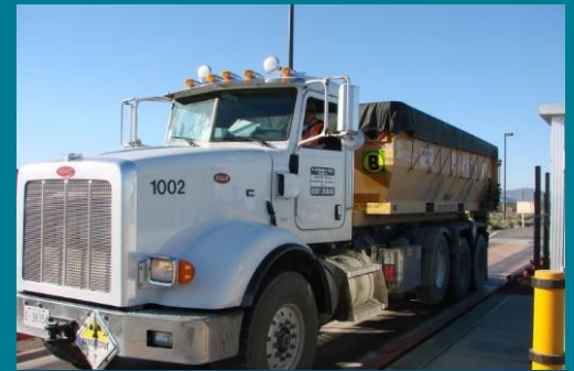
Environmental Restoration Disposal Facility containers are weighed and characterized to track contents of waste.
